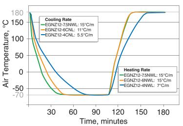
Different Global-N models can heat and cool at different rates. Shown above are change rates for EGNZ12 models, following IEC 60068 3-5 standard, with the sensor in the supply air.
