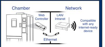
The Web Controller is compatible with all USA-built ESPEC models with touch-screen programmer/controllers, except thermal shock.
