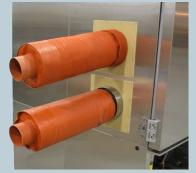
Allows conditioning of remotelylocated equipment that cannot be placed inside the chamber.
